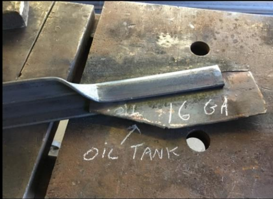
Gap for Galvanization
